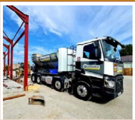
Volumetric Truck Delivering precise amount of concrete to your door
